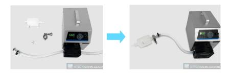
**d.** Open the pinch valve by turning it counterclockwise.
