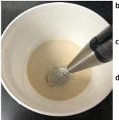
b. Add the Nanostabilizer®-LSO and distilled water pre-mix into the storage tank. Use the silicone spatula to ensure that the entire pre-mix is added to the storage tank.
