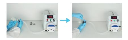
**b.** Using your pump at a flow rate setting of 100 - 150 ml/min, sterilize the nanoemulsion by passing it through the in-line filter into the presterilized finished product container.
