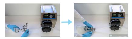
**b.** Using your pump at a flow rate of 250 - 300 ml/min, sterilize the nanoemulsion by passing it through the in-line filter into the presterilized finished product container.
