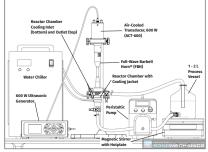
liquid recirculation network are properly clamped. The distilled water should be set up to flow from the bottom of the process vessel to the reactor chamber and back to the top of the process vessel (see LSP-600 User Manual and LSP-600 Peripheral Assembly Equipment Guide for details). To avoid foaming, make sure that the hose returning the liquid to the process vessel is submerged into the liquid by about 5 cm.
