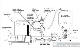
Dispense  $\mathbf{9}$  L of distilled water into the storage tank with mixer. Start running the mixer at a high speed (80 – 100 %).
