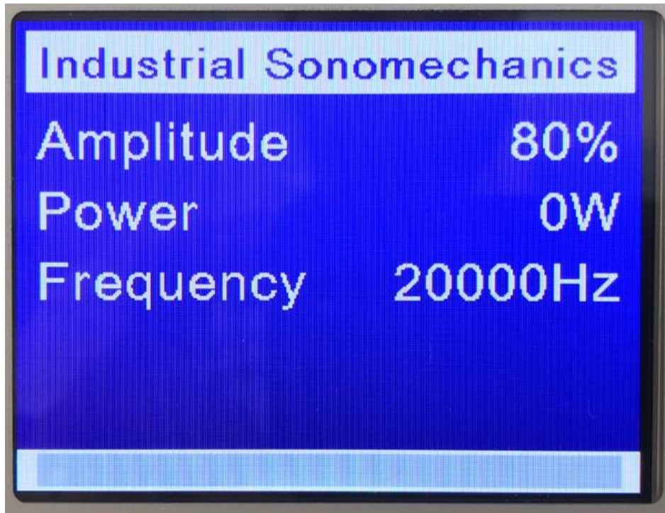
Figure 3 – 8. The LSP-600 generator’s LCD display.
