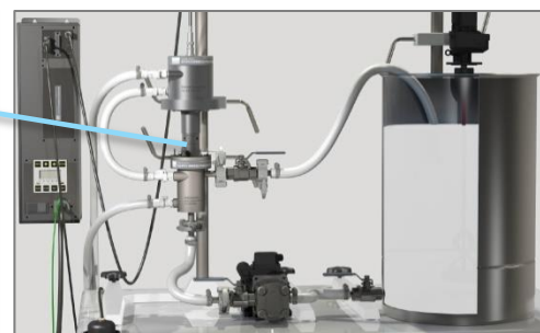
Figure 1c. BSP-1200 in flow-through mode using a Half-wave Barbell Horn (HBH).
