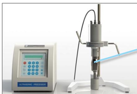
Figure 1a. LSP-500 in batch mode using a conventional horn (CH).
